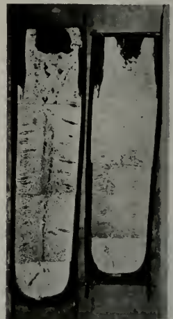
The specimen on left shows the resultant pockets of porosity that may develop when dissolved hydrogen is not permitted to escape from steel while being cast. Such pockets can easily ruin an entire heat of steel. Application of a flushing process, developed by AIR REDUCTION Sales Company engineers, by which dry nitrogen or argon is bubbled through the metal, eliminates the dissolved hydrogen efficiently and at a reasonable cost. The specimen on the right clearly shows the results obtained when the Airco flushing process is used.
